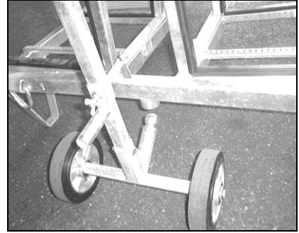
Picture 5.6 – Transport by using the pole
